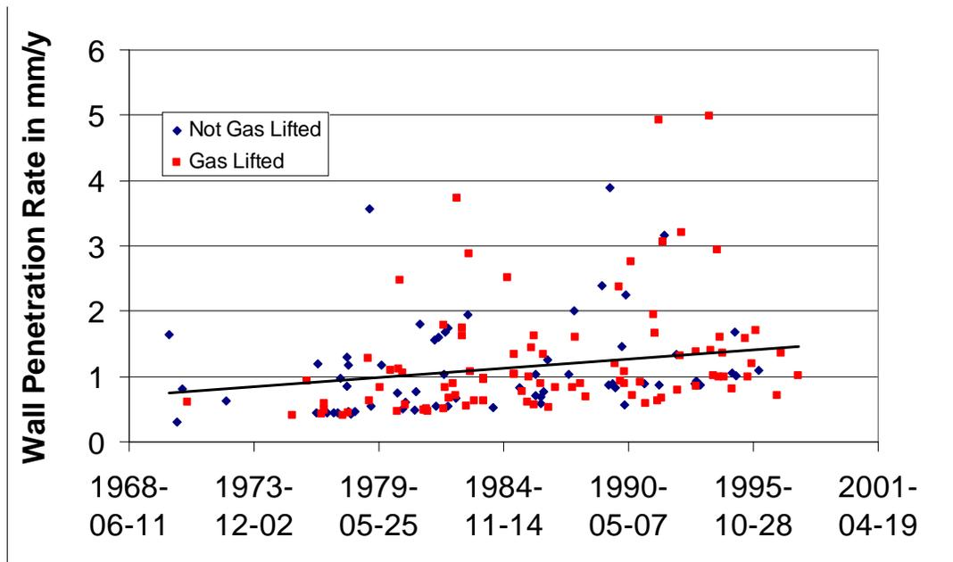
**Figure 5: The production casing corrosion rate as a function of well completion date. Red symbols are wells with gas lift and blue symbols are naturally flowing producers and injectors.**
