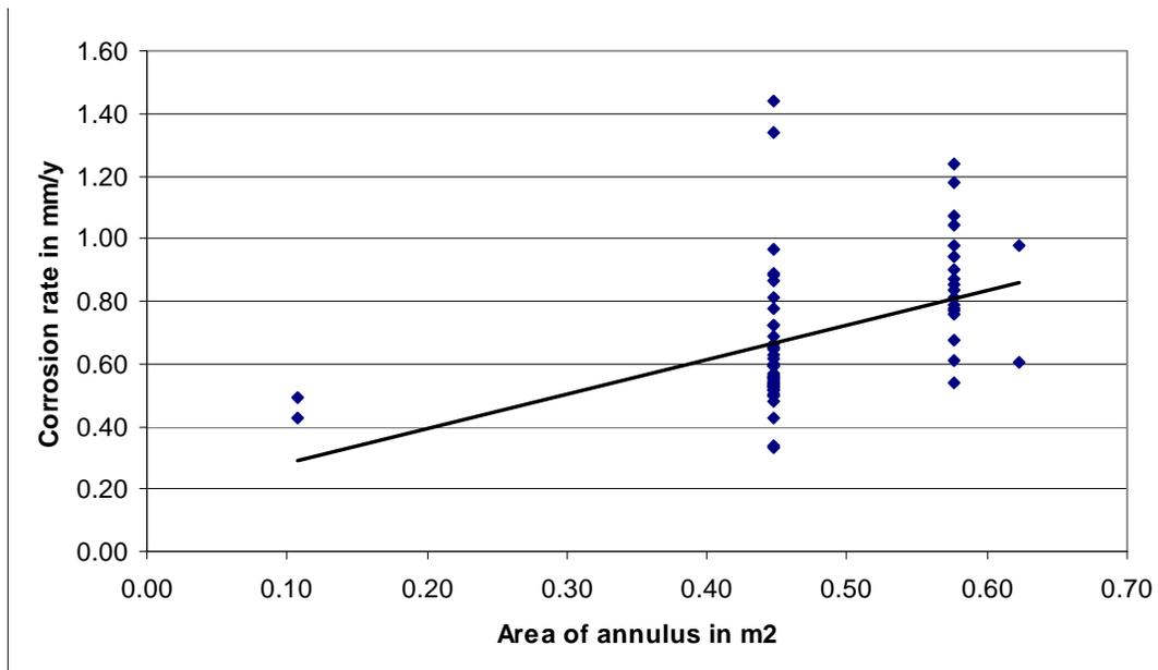
**Figure 3: Surface Casing corrosion rate as a function of annulus cross sectional area.**
