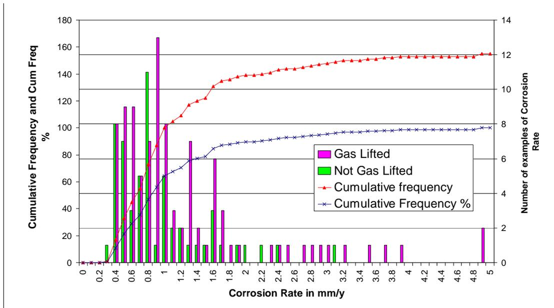
**Figure 4: Histogram of apparent production casing corrosion rate identifying the gas lifted wells. The cumulative frequency is the sum of the total number of failures of all wells. The cumulative percentage shows, for example that approximately 80% of the failures arose at corrosion rates less than 1.5 mm/y.**
