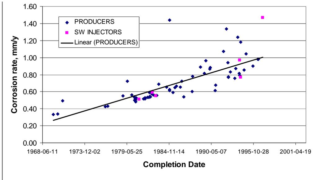
**Figure 1: Distribution of Surface Casing corrosion rates experienced within 72 failures including 6 seawater injector wells.**
