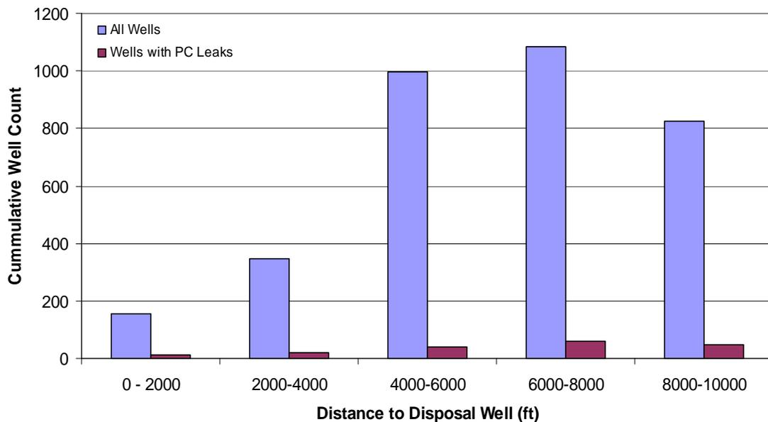
**Figure 7: This is a count of all wells at the stated distances (extracted at the depth of leaks) from the disposal wells compared to the numbers of wells with identified production casing (PC) leaks.**
