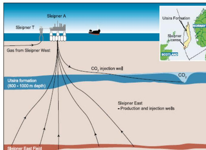
**Figure 1 : Simplified diagram of the Sleipner CO<sub>2</sub> Storage Project. Inset: location and extent of the Utsira formation.**
